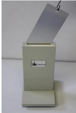
In order to be able to also determine the quantity of coating on the aluminium an analytical method was developed in which an aluminium test plate is immersed, after treatment, in a stripping cuvette in order to remove the coating.
